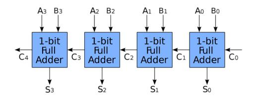
The layout of ripple carry adder is simple, which allows for fast design time; however, the ripple carry adder is relatively slow, since each full adder must wait for the carry bit to be calculated from the previous full adder.
