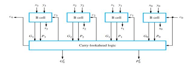
$P_i$  is called a carry propagate because it is term associated with the propagation of the carry from  $G_i$  to  $C_{i+1}$ . Now  $C_{i+1}$  can be expressed as a sum of products function of the P and G outputs of all the preceding stages.
